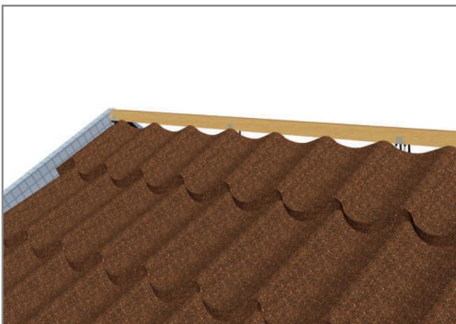
**Fig 9.2.1** Tile adjoining to the ridge batten
