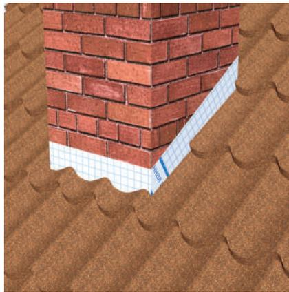
Fig 9.5.2 Tile installation in the place of adjoining
