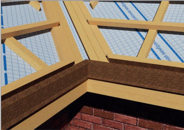
Fig 8.6.3 Eaves flashings
