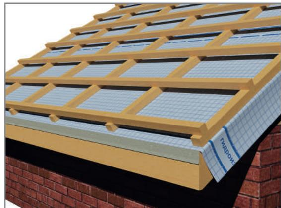
Fig 8.4.2 The roof sheathing without rainwater hooks
