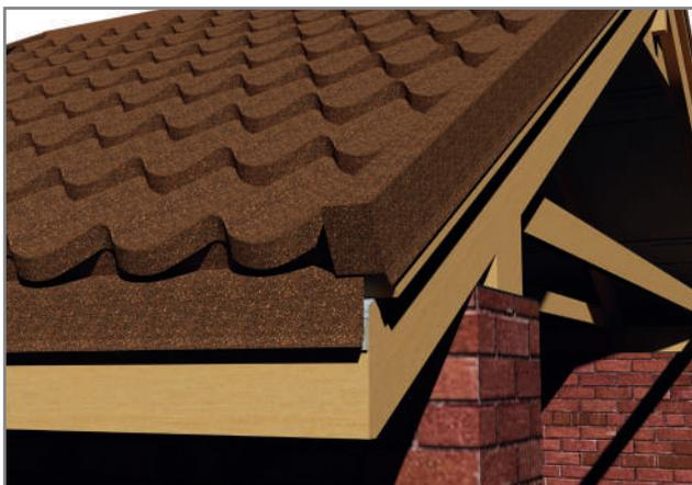
Fig 9.4.5 The gable board with ending cap installation
