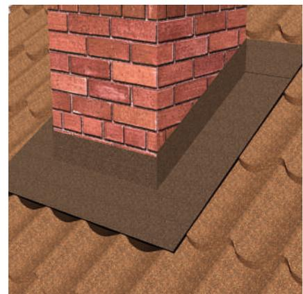
Fig 9.5.6 Side flashing installation at the side and top of adjoining node
