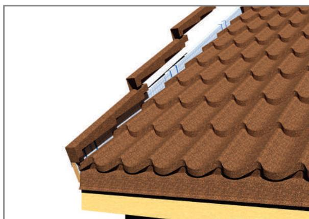
Fig 9.4.2 Gable flashing installation
