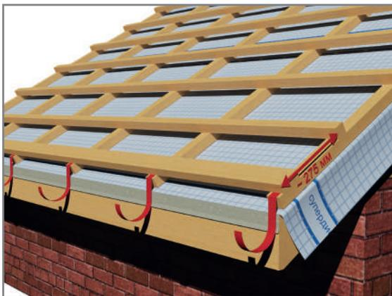
Fig 8.4.1 The roof sheathing with rainwater hooks
