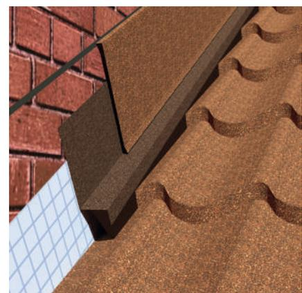
Fig 9.5.8 The adjoining of roof pitch to the wall parallel to the slope
